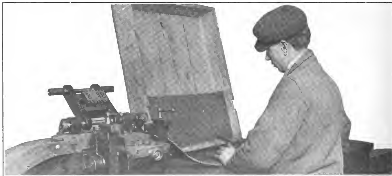
Stage 3—Cutting the clamped tubes to their proper length and placing them in a box of the correct width
